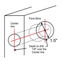
6 - Apply the Screw Bracket on to the Latch Bolt from the exterior side; and install the assemblage into the door edge bore
