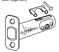
9 - Apply the Tail Piece into the T turn slot; install the T Turn set with the engaging the Tail Piece onto the Latch Hub. Test the lock function and fasten the T Turn set with Bolting Screws x 2 (measure the Screw and cut in proper\_length)
