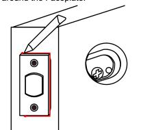
7 - Apply the Faceplate and fasten with wood screws x 2
